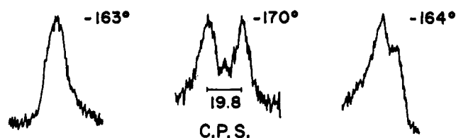
Figure 1. Bands of H-4 and H-5 in cyclohexene- cis -3,3,4,5,6,6- d 6 in bromotrifluoromethane solution at low temperatures.
